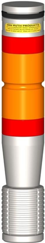
CEMENTING AND WEDGING BOTTOM PACKERS (CWBP) are used for cementing, wedging, and isolating ore zones or in conjunction with Sub Set Grout Packers (SSGP) to pressure grout specific fault zones or with permeability testing to isolate previously tested zones. They are also used in place of the Cementing Wedging Plug (CW) for applications where controlling water ingress is required.
