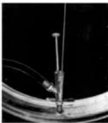
Tire rotated so valve is at bottom with hydroinflation fluid being removed.
