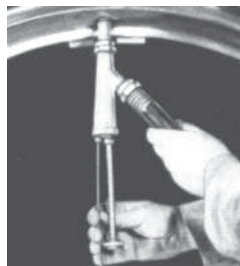
Tire being filled with hydroinflation equipment.
