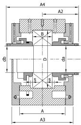
Housing - Flame-Cut Steel End Covers - Flame-Cut Steel
