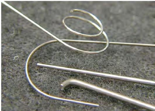
Figure 4: Examples for formed parts of Nitinol fabricated by constraint thermal shape-setting process.
